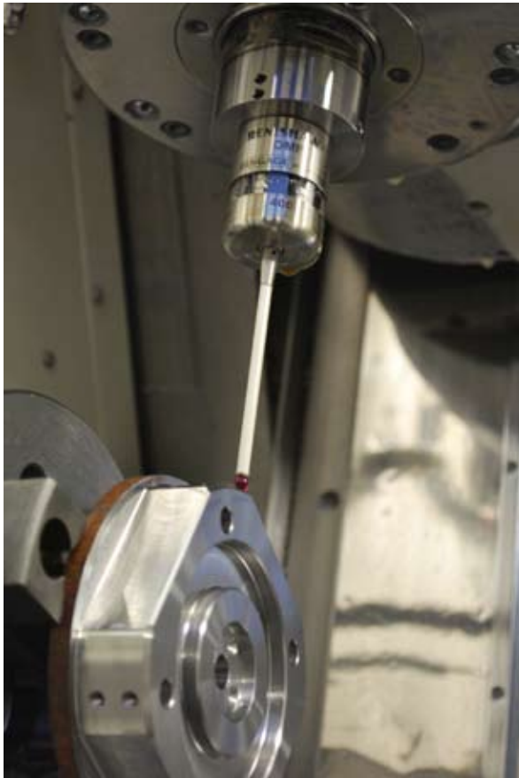
Mazak Integrex multi-axis mill-turn machine with Renishaw OMP400 in the spindle
